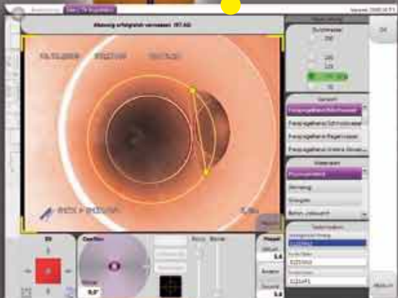
Determining the nominal diameter of branch pipes
